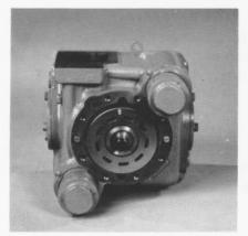
Place the pump horizontally in preparation for removal of the cylinder block assembly
