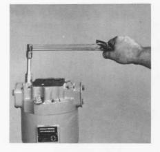
Install two (2) end cap screws and alternately tighten them until the internal spring has compressed far enough for the end cap to rest on the housing. Install the remaining screws.
