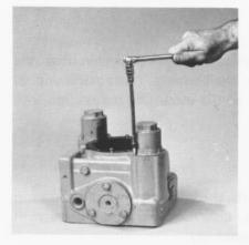
After adjustment has been completed, the retainers can be installed and peened into the locking slot on the housing.
