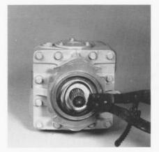
It is recommended that all shaft seal parts be replaced. If parts are to be reused, they must be protected from being damaged by the shaft during removal.
