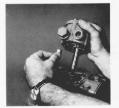
To remove the charge pump, loosen the four (4) cap screws that form a rectangular pattern on the rear of the charge pump. Do not remove the screws at the top and bottom as these hold the segments of the charge pump together.
