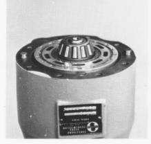
Install the bearing plate so that the milled slot locates over the pin and the pilot ring fits in the center bore of the cylinder block. After installation lubricate the exposed surfaces with clean hydraulic oil.
