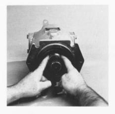
The bronze sealing ring is also held in place by internal O-ring friction. Work this part free and carefully slide over the shaft.
