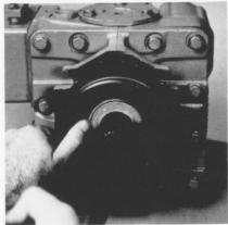
Install the retaining ring with the beveled side out, putting the side opposite the tangs into the groove first. Be certain that the retaining ring has snapped into its groove completely.
