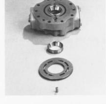
The end cap is actually an assembly consisting of a tapered bearing race which is a slip fit in the end cap and the valve plate locating pin. These parts should be removed from the end cap. There may or may not be a shim located under the bearing race which should be removed.
