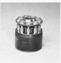
If the cylinder block assembly does not remain together during removal, it can be easily reassembled at a later time.
