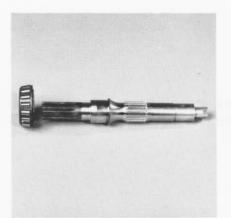
The tapered bearing can be pressed off the shaft if required. Be careful not to damage the seal diameter of the shaft while removing the bearing.
