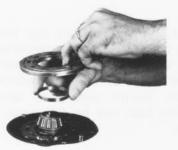
Install the pilot ring and the locating pin in the cylinder block.
