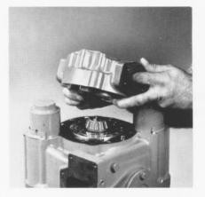
Install the end cap and valve plate, holding the valve plate so it does not drop off during assembly.
