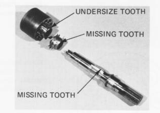
Lubricate the thrust plate, slippers, pistons, and bores with clean hydraulic oil. While holding the shaft on the external end, align the missing tooth of the shaft and ball guide by sighting through the control cavity. Using the locating pin hole as a guide, slide the cylinder block assembly onto the shaft and against the thrust plate. When properly installed a spring load can be felt when pushing against the cylinder block.
