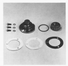
Be certain to keep the plastic shims with the proper trunnion to insure satisfactory bearing adjustment after reassembly.
