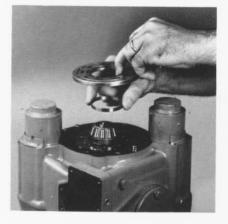
Install the pilot ring in the bearing plate and the locating pin in the cylinder block. Install the bearing plate so that the milled slot locates over the pin and the pilot ring fits in the center bore of the cylinder block. After installation, lubricate the exposed surfaces with clean hydraulic oil.
