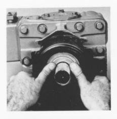
Insert the stationary seal pilot into the aluminum housing, locating the notch in the stationary seal over the pin in the housing.
