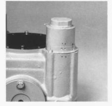
First, mark the servo housing for location to the pump housing. This set of marks should line up to show the rotational position of the servo housing to the pump housing.
