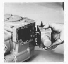
Engage the pin on the control link in the mating hole in the small link attached to the swashplate.
