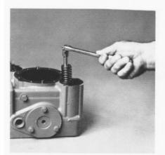
Do not reuse the screw holding the spring to the servo piston as it has a nylon locking insert that is not effective when reused. These springs should not be removed unless necessary.
