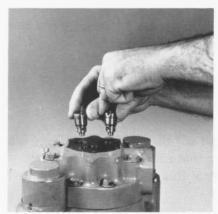
The removal of the charge check valves requires the use of a drag link socket.
