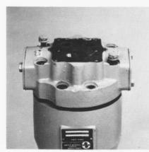
There is an internal spring loading on the end cap and as the last two (2) screws are loosened, it should begin to separate from the housing. Loosen these screws alternately until the end cap has fully separated from the housing, then remove the screws entirely.
