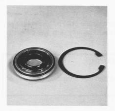
Insert the stationary seal pilot into the aluminum housing, locating the notch in the stationary seal over the pin in the housing.
