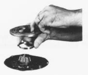
If the pilot ring remains with the bearing plate, remove it at this time.
