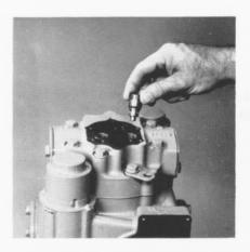
Use caution when installing these valves to prevent damage to the O-ring on the cartridge as it is inserted past the threads. Lubricate O-rings before installation.
