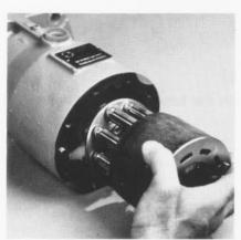
Place the motor in a horizontal position. Slide the cylinder block assembly off the shaft while holding the external end of the shaft.
