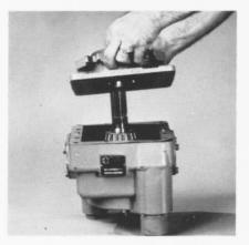
Set the pump on the servo housings and remove the front cover screws.
