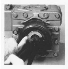
Install the remaining major assemblies (Control Valve, Check Valves and Charge Pump) as outlined in the Minor repair procedures.
