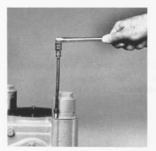
Remove the locking retainers using a 12 point, 3/16 socket for the cap screws.
