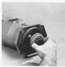
Remove the housing from the shaft. This part is actually an assembly that is being held together by the friction of an internal O-ring. It will normally remain assembled until physically separated.
