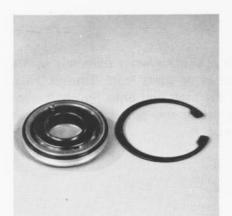
Remove the housing from the shaft. This part is actually an assembly that is being held together by the friction of an internal O-ring. It will normally remain assembled until physically separated.
