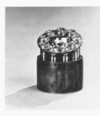
The cylinder block assembly usually comes out in one piece; however, some of the parts can separate. This does not present a problem as these parts can be reassembled later.
