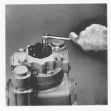
Remove charge pump and control valve as outlined under Minor repair procedures.
