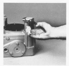
Unscrew the servo housings using channellock pliers to grip the flats on top of the housings.
