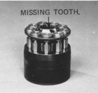
To install the cylinder block assembly, it is necessary to check the alignment of certain parts. There is no special relationship of pistons to bores, springs, etc.. However, the alignment of the ball guide and cylinder block splines is critical. The undersized tooth in the spline of the cylinder block must line up with the missing tooth in the ball guide spline.
