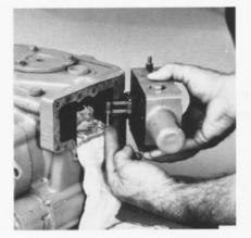
Install the connecting pin through the control linkage and the feedback link on the swashplate with the headed side toward the center of the pump. Use caution not to drop parts into the pump housing.
