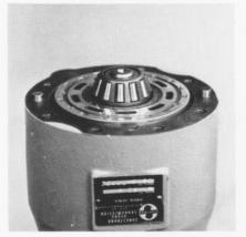
Remove the bronze bearing plate and pilot ring from the cylinder block.
