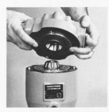
Place the end cap gasket on the housing, being certain the locating pins are in place, then install the end cap and valve plate. Hold the valve plate so it does not drop off during assembly. The end cap and gasket will only align with housing mounting holes in one position.
