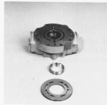
Assemble the bearing race, shim (if required) and locating pin in the end cap. Check the valve plate to be certain it is a pump valve plate (has 2 tapered slots) and that it is for correct rotation (slots point away from direction of rotation).
