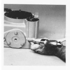
The trunnions should be marked to insure reassembly to the correct side of the housing.
