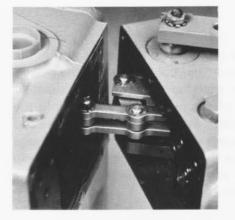
Swing the control away from the housing as far as it will go to expose the cotter pin.
