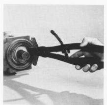
It is recommended that all shaft seal parts be replaced. If parts are to be reused, they must be protected from being damaged by the shaft during removal.
