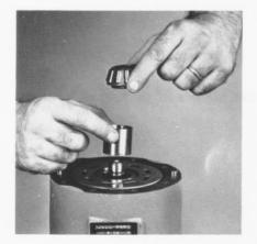
After removal of the bearing, slip the spacer out of the bore in the cylinder block.
