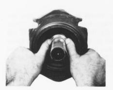
Before installing any shaft seal parts, wrap the shaft with a protective covering to protect parts from damage. Then slide the sealing ring over the shaft and onto the shaft pilot diameter with the O-ring facing the motor. Work the ring into place using hard force only.
