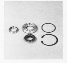
Prior to assembly, place one O-ring in the I.D. of the bronze sealing ring and one O-ring in the I.D. of the aluminum housing. Place the six (6) or more springs in the cavities in the housing. Care must be used to protect the parts from damage by the shaft during assembly.
