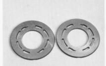
The valve plate on the left in the picture is for Left Hand (CCW) rotation. The valve plate on the right is for Right Hand (CW) rotation.
