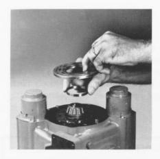
Remove the bronze bearing plate and the pilot ring from the cylinder block. If the pilot ring remains with the bearing plate, remove it at this time.
