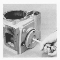
Friction caused by the O-ring on the trunnion may make it necessary to use a slide hammer to pull the trunnion assembly.
