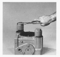
Slide the housing over the servo piston and thread it into the pump housing.
