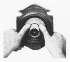
Install the O-ring on the O.D. of the housing then slide it into place against the bronze sealing ring. Since this is a spring loaded assembly, it may be necessary to push against the aluminum housing to expose the retaining ring groove.
