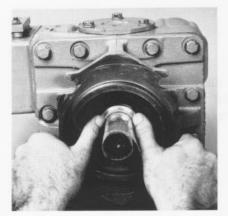
Before installing any shaft seal parts wrap the shaft with a protective covering to protect all parts from damage. Then slide the sealing ring over the shaft and onto the shaft pilot diameter with the O-ring facing the pump. Work the ring into place using hand force only.
