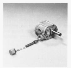
The charge relief valve can be inspected by removing the hex. plug, spring and poppet. Remove the shims from the counterbore of the hex. plug. Do not alter these shims unless new parts are used, in which case the valve must be re-shimmed to the proper setting.
