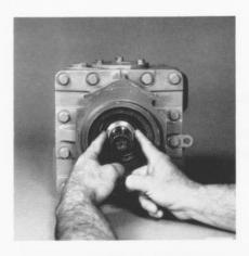
The bronze sealing ring is also held in place by internal O-ring friction. Work this part free and carefully slide over the shaft.
