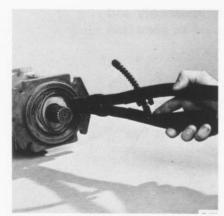
Remove the shaft seal as outlined under Minor repair procedures. The shaft seal must be removed before end cap screws are loosened to prevent the seal being damaged.
