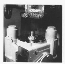
The tapered bearing should be installed with an arbor type press for the most satisfactory results. This bearing can not be driven onto the shaft due to the internal spring loading of the cylinder block and shaft. Press on the inner race of the bearing and use care not to damage roller cage.
