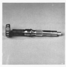
The tapered bearing can be pressed off the shaft if required. Be careful not to damage the seal diameter of the shaft while removing the bearing. The bearing race is press fit in the housing. If any of these parts are replaced, the shaft end play must be checked.
