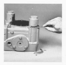
After removing the retainers, scribe a line to mark the height of the servo housing in relation to the pump housing.
