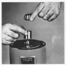
Set the motor vertically and install the spacer in the center bore of the cylinder block.
