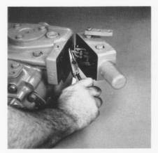
Remove the cotter pin, washer and connecting pin. It is suggested that a piece of wire be inserted through the eye of the cotter pin so the pin can easily be retrieved if it falls into the pump.
