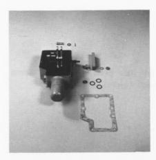
In preparation for reinstalling the control, place a new gasket on the housing, and place the orifice plate and O-rings in the control.
