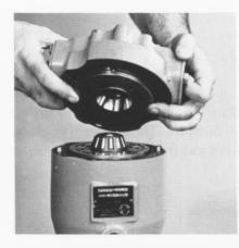
The end cap can now be lifted off the motor; however, be certain that the valve plate does not fall and become damaged. If the valve plate tends to lift off with the end cap, hold it in place on the end cap and remove both parts together. If the valve plate remains on the bearing plate, remove it at this time.
