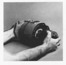
Lubricate the swashplate, slippers, pistons and bores with clean hydraulic oil. Hold the shaft on the external end, align the missing shaft tooth with the missing ball guide tooth using the locating pin hole as a guide. Slide the cylinder block assembly onto shaft and against swashplate face. When properly installed a spring load can be felt when pushing against the cylinder block.
