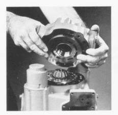
The end cap can now be lifted off the pump; however, be certain that the valve plate does not fall and become damaged. If the valve plate tends to lift off with the end cap, hold it in place on the end cap and remove both parts together. If the valve plate remains on the bearing plate, remove it at this time.
