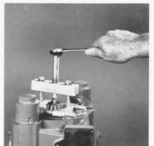
The tapered bearing must now be removed from the shaft. A bearing puller should be used that will pull against the inner race of the bearing. A spacer is required to protect the slot in the end of the pump shaft from the puller screw. Protect the face of the cylinder block during this operation.
